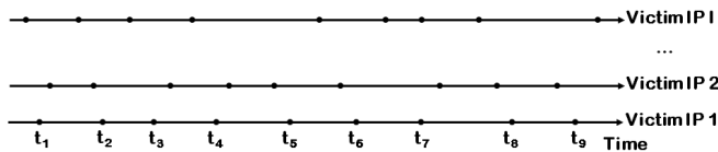
(a) Illustration of victim-level stochastic cyber attack processes with respect to individual victim IP addresses, where dots represent attack events and (for example) attacks against victim IP 1 arrive at time t_1, \dots, t_9 .
